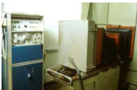
A 'step and repeat' camera showing a paper tape system for positioning each image correctly.
